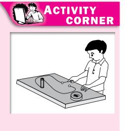
Repeat the experiment a few times, you will notice that the needle deflects when the current is switched on and stays in that position as long as the current flows in the wire. When the current is switched off, the needle comes back to its original North-South direction.
